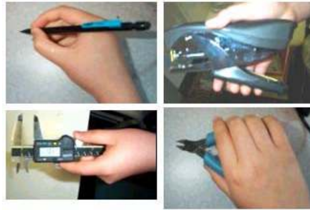
Figure 17. Precision grip uses the index finger to position an object (left). Strength grip uses all fingers in tandem (right).
