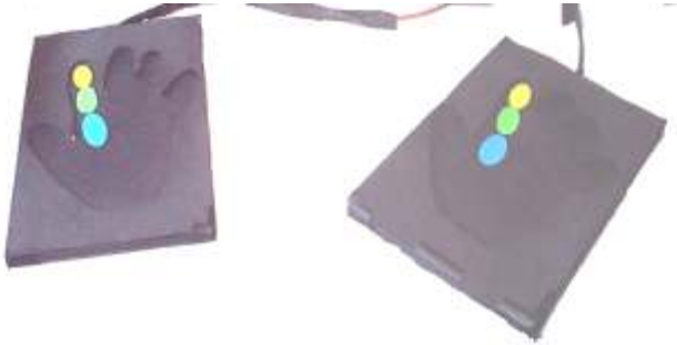
Figure 7: ComTouch preliminary implementation. One-finger of vibrotactile communication is conveyed between two pads.
