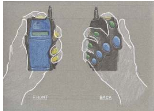
Figure 1. ComTouch Concept drawing showing a handheld sleeve that fits onto the back of a mobile phone
