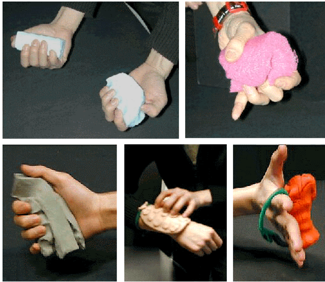
Figure 5: Exploration of different form factors using rough prototypes made from clay, foam and wire.
