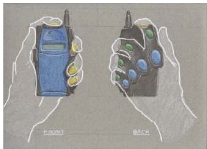
Figure 18. ComTouch concept drawing depicts the ergonomic grip.
