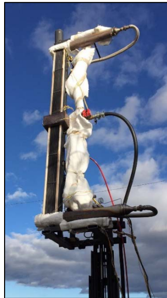
Figure 33. A pair of absorber modules, mounted one atop the other. Inlet flow enters in the middle and distributes up and down through the modules.
