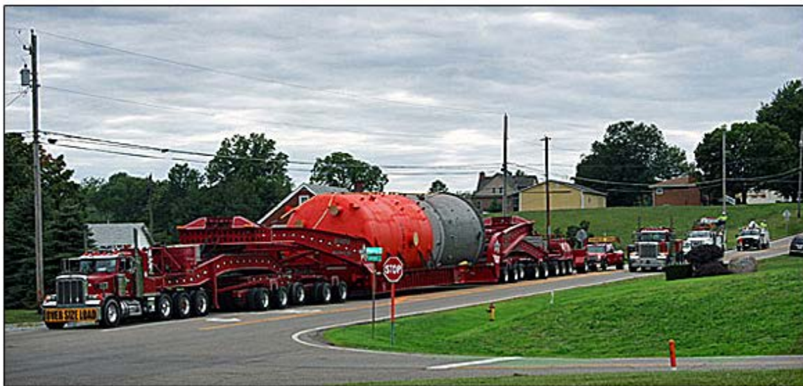
Figure 51. 180-in. diameter x 60-ft long (4.5-m x 18-m), 90-ton pressure vessel manufactured by Halvorsen for the petrochemical industry [www.halvorsenusa.com].
