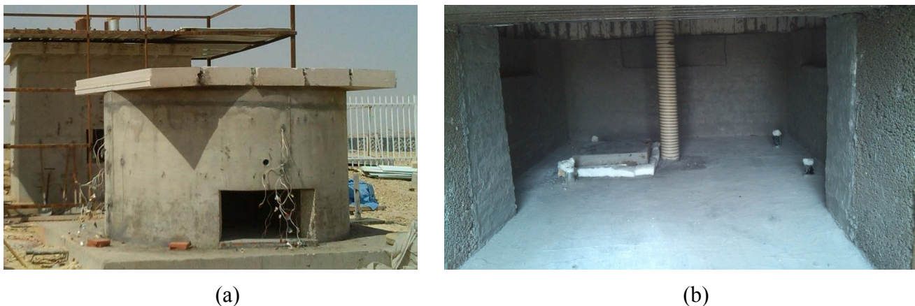
Figure 22. Ground-based cylindrical TES test facility, (a) overall view of the cylindrical TES bin, (b) the electric heater inserted along the centerline of the TES bin to artificially heat the particles for heat-loss testing.
