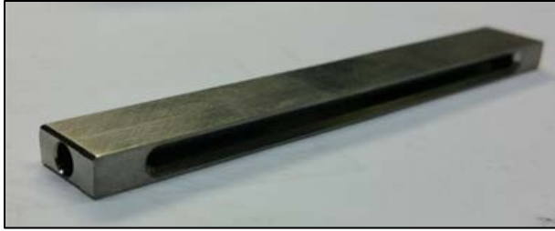
Figure 31. Example manifold block, which is used to cap the unit cell.
