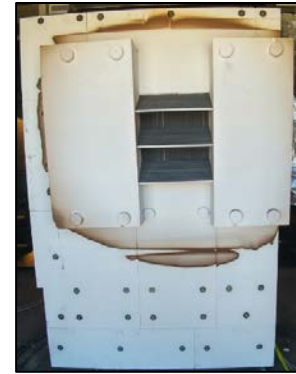
Figure 45. Bladed receiver in place after on-sun testing.
