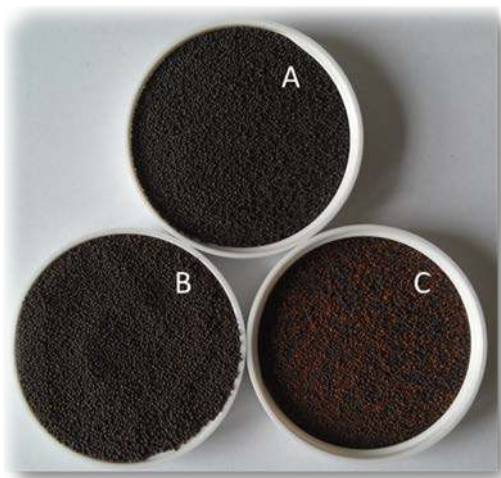
Figure 16. Spherical ceramic particles provide high solar absorptance and durability.
