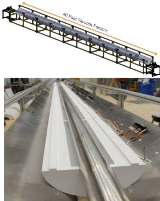
Figure 40. Vacuum furnace to enable the fabrication of high length/diameter heat pipes with lengths approaching 40 feet.
