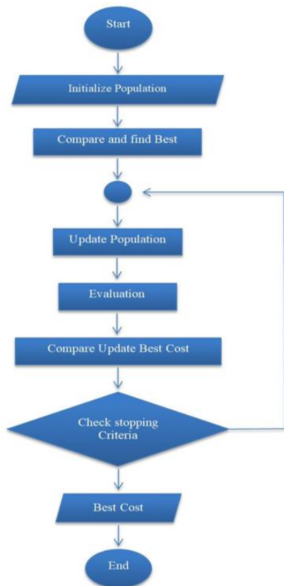
Figure 2. Flow chart of genetic algorithm
