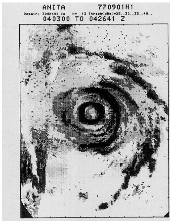
FIG. 3. Composite of digital radar reflectivity data observed in Hurricane Anita during passes 13 and 14 of Fig. 2b. Figure represents an area 300 \times 400 km. (This and other radar imagery were prepared by Dave Jorgensen and Frank Marks of NHRL.)
