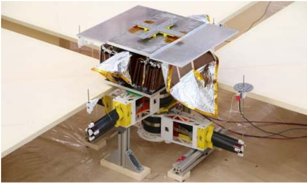
Fig. 12 Deployment test breadboard setup (2 boom deployment units with 2 booms each and one PV blanket stowed in storage box)
