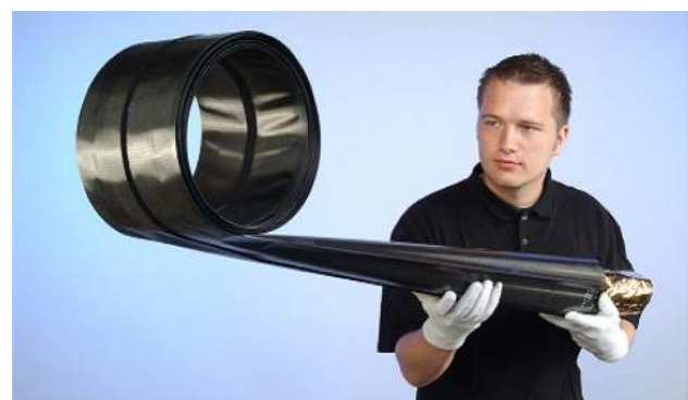
Fig. 8 DLR’s tubular, reelable boom in partially deployed state
