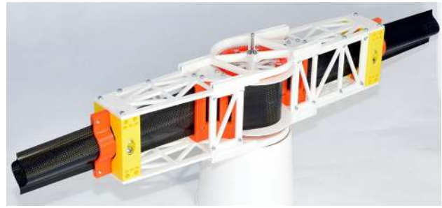
Fig. 10 Breadboard model of a single deployment unit with two opposing booms reeled on a central drum
