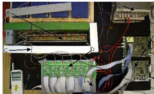
Figure 6: Picture of the measurement setup with (A) the module ladder (half-stave) with six serially powered modules containing about 0.3Mpixels, (D) AC coupling read-out and power routing board, (E) constant current power supply, (F) pixel read-out electronics
