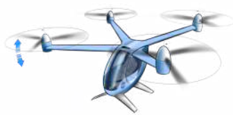
Figure 1. Single-passenger quadrotor with electric propulsion.
