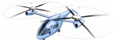
Figure 2. Six-passenger side-by-side helicopter with hybrid propulsion.
