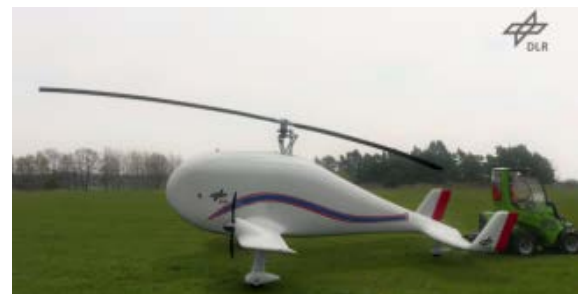
Fig. 1. DLR ALAADy – Automated Low Altitude Delivery – Animated gyrocopter-version. Source: DLR
