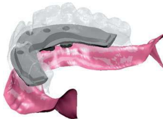
Figure 12 CAD implant framework with a modified I-bar design. The apical buccal and lingual portions of the framework were designed for use as finish lines for the denture base portion of the hybrid prosthesis.
