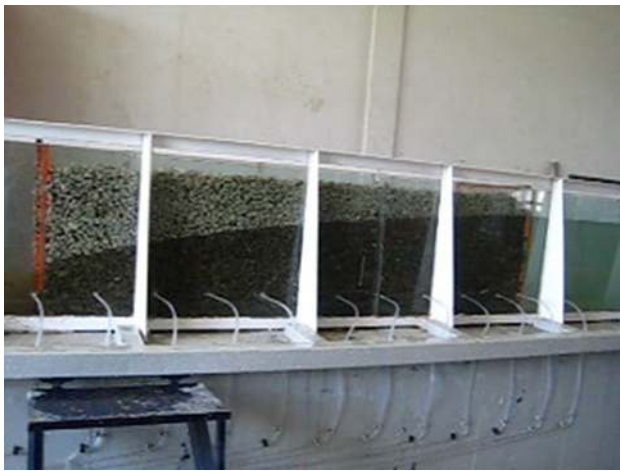
Fig. 2 Experimental setup containing a packed medium through which phreatic line can be seen
