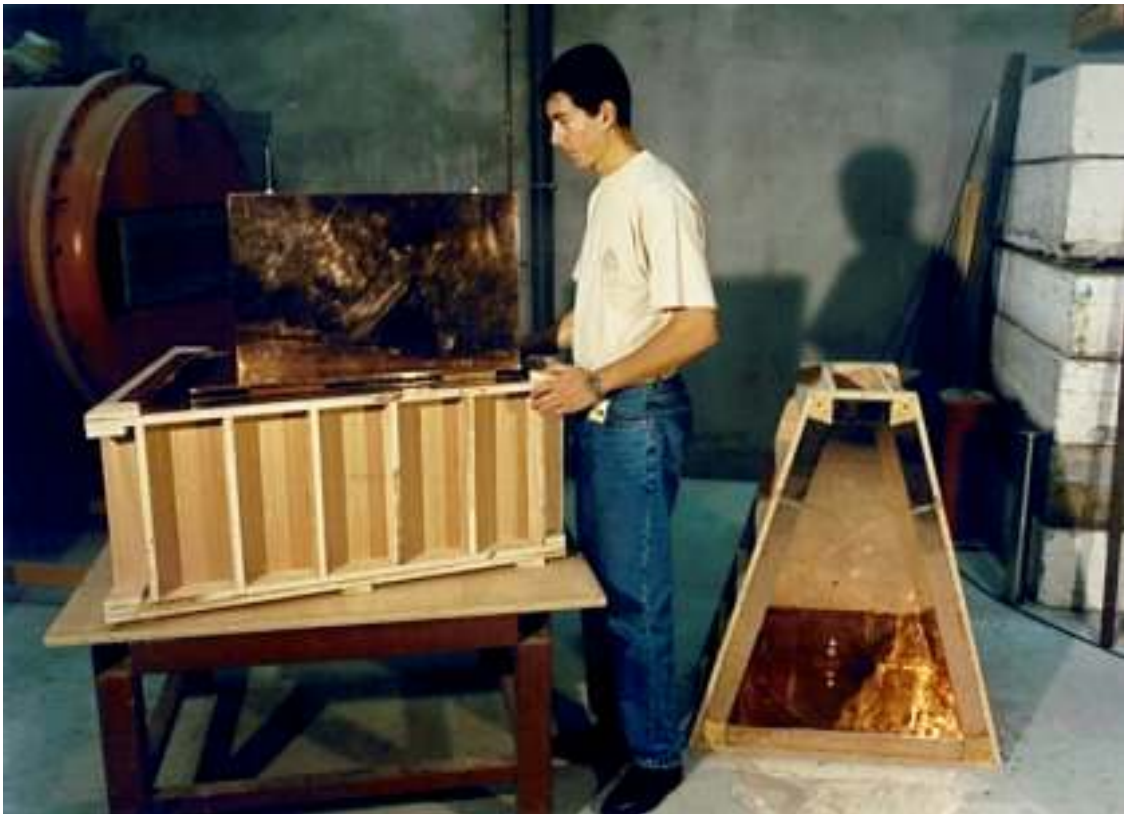
FIG. 3.5 Photographs of the cavity models (top : flat-topping cavity during assembling ; bottom : main cavity during assembling.)
