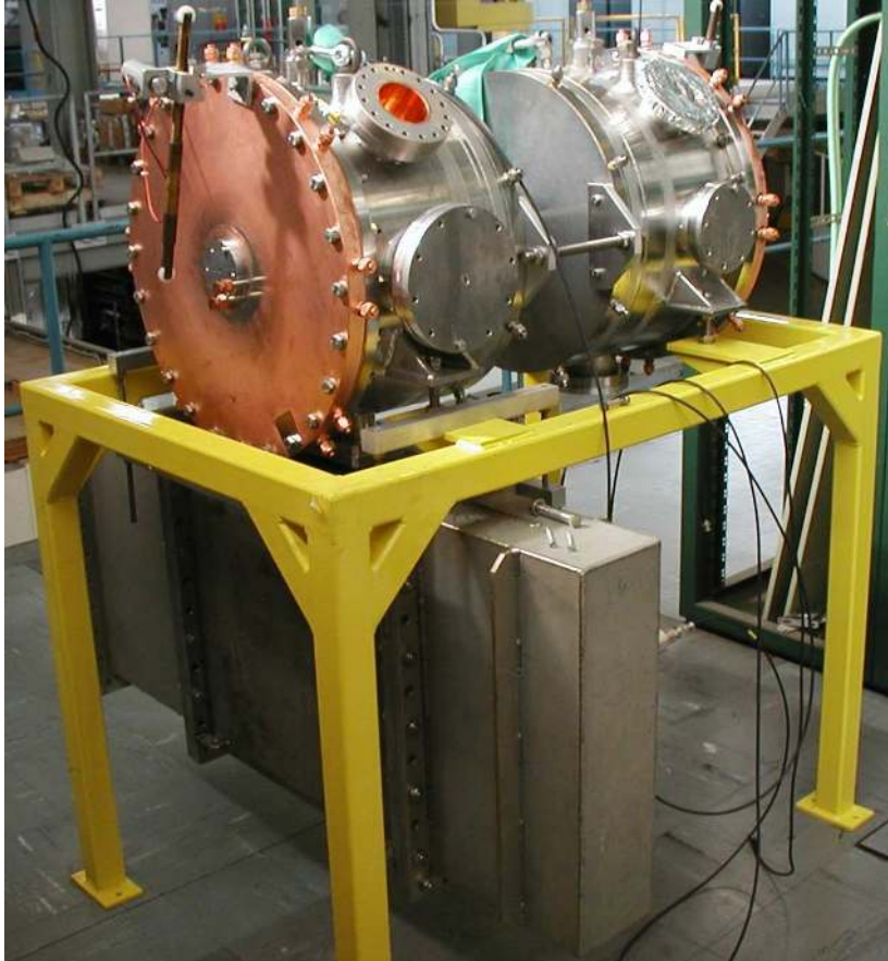
Fig. 4.19: The CERN CCDTL prototype including power coupler at the bottom during low-level RF tests
