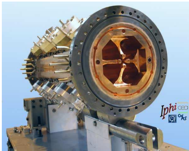
Fig. 4.3: One of six modules of the IPHI RFQ
