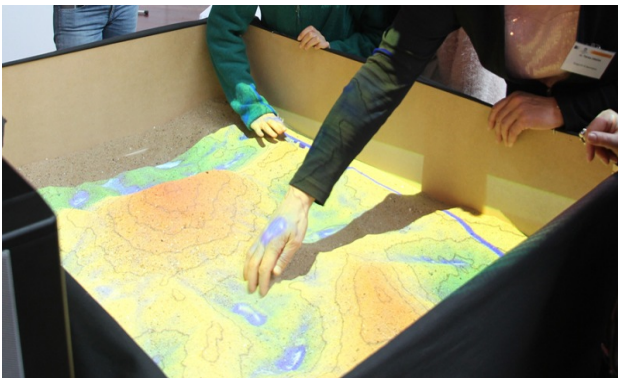
Figure 4. Water flow simulation by Simulation Augmented Reality Sandbox (Courtesy of B. D. Vlieghe Dr. C. Stal, Ph. de Mayer, Gent University, Belgium).
