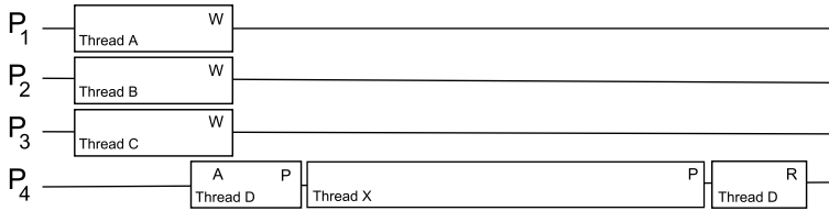
Figure 1.8: The active thread on processor P_4 acquires the lock. P_1 , P_2 , and P_3 also need the lock to be able to proceed. The thread on P_4 that holds the lock is preempted by another thread before it can release the lock. All threads are now waiting for a thread that does not even use the lock.
