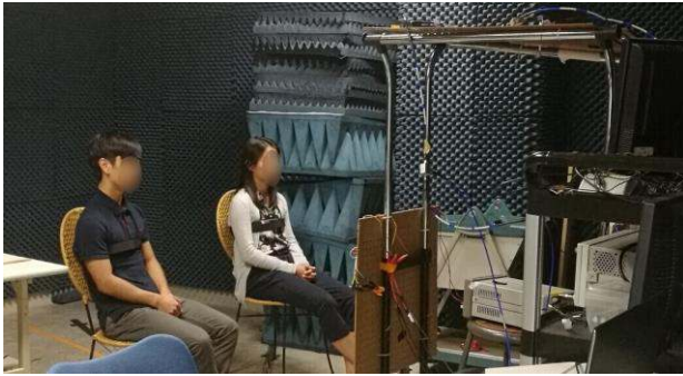
FIGURE 3. Experimental setup showing two well-spaced subjects. These subjects can be separated using DOA and respiration rate of each independent subject can be monitored by tilting the radar beam in the corresponding angular direction.
