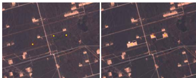
Figure C4. Example of an area where new development was found, before (left) and after (right) shown in Sentinel-2 imagery (ESA, 2020). Points in yellow indicate the locations of new well pad development.
