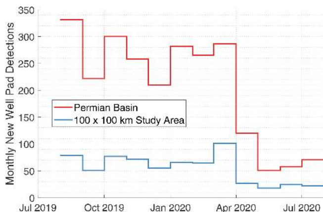
Figure 7. Number of new well pads constructed per month between 1 August 2019 and 31 July 2020 in the full Permian Basin and our 10 000 km 2 Delaware subsbasin study area based on satellite imagery and machine learning (Appendix C).
