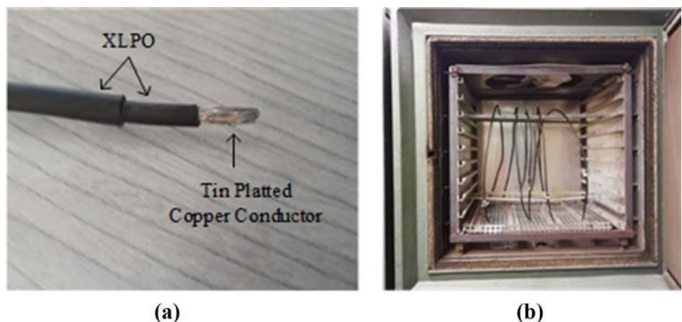
Fig. 1 a Low voltage power cable sample under investigation; b Air circulating oven for thermal aging
