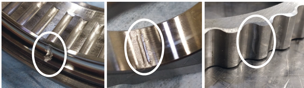
FIGURE 3: Gearbox artificial damages.
