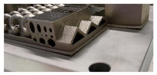
Figure 7. Example of layer delamination [30].
