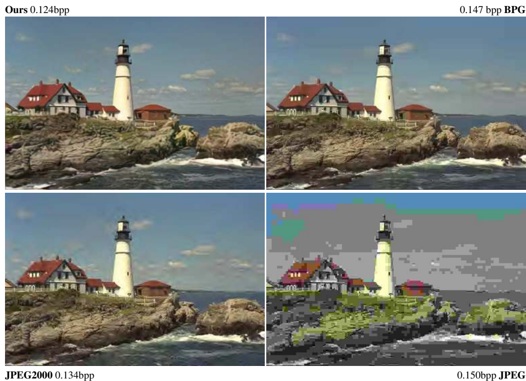
Figure 5: Example image ( kodim21 ) from the Kodak testing set, compressed with different methods.
