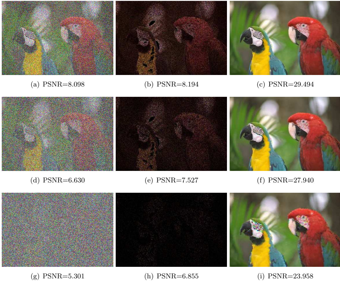
Figure 12: Example of noise removal by proposed method.(a)-(c) Experiment (50%). (d)-(f) Experiment (70%). (g)-(i) Experiments (95%). First column shows images contaminated by marginal salt-and-pepper noise, second column includes mask image by using Eq. (14) and third column displays the result of the conditional toggle mapping.
