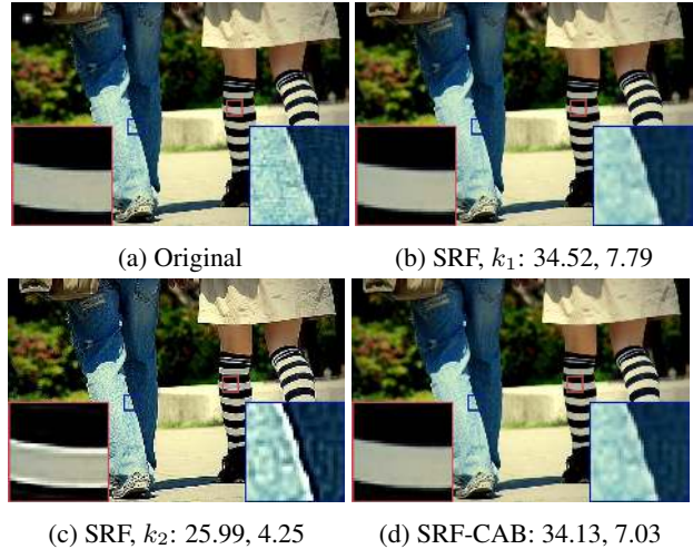
Figure 4: (a) depicts the high-resolution image h . The corresponding low-resolution image l was created with k_1 (top left corner). (b-c) show the up-sampling result obtained by the SRF, which was trained on k_1 and k_2 , respectively. (d) presents the result of our proposed conditioned SRF. The image is taken from [24] and the upscaling factor is 2.
