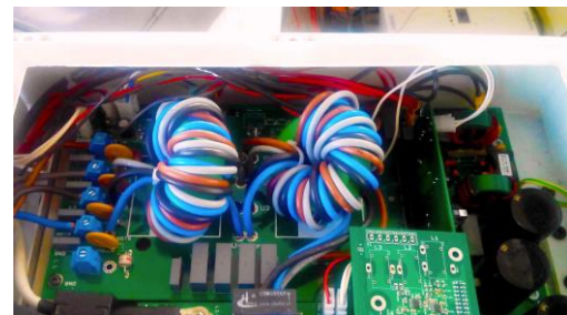
FIGURE 20. Designed EMI filter 2 for PV inverter.
