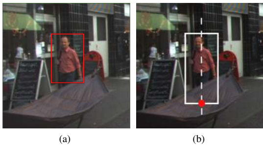
Figure 5. The detected 2D bounding box (a) is corrected using the back-projected foot point from 3D (b).
