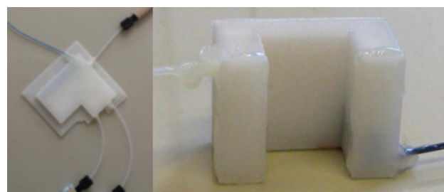
Fig. 6 Physical set-up of the 3D-printed reactionware used in the polyoxometalate syntheses. (Left) Three inlet device (R2) used with inlets of \text{Na}_2\text{MoO}_4 \cdot 2\text{H}_2\text{O} , \text{HCl}_{(\text{aq})} and \text{NH}_2\text{NH}_2 \cdot 2\text{HCl} . (Right) One inlet device (R3) where HCl is flowed through silos containing solid \text{Na}_2\text{MoO}_4 \cdot 2\text{H}_2\text{O} and hydrazine dihydrochloride, respectively.
