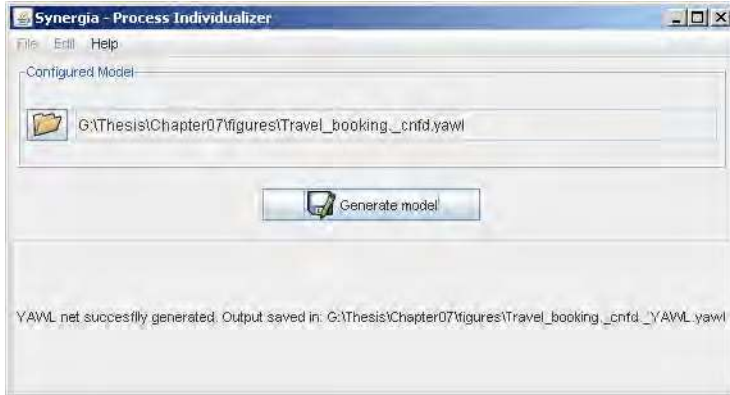
Figure 5.10: The Process Individualizer generates a classical process model according to the configuration decisions provided in the model.
