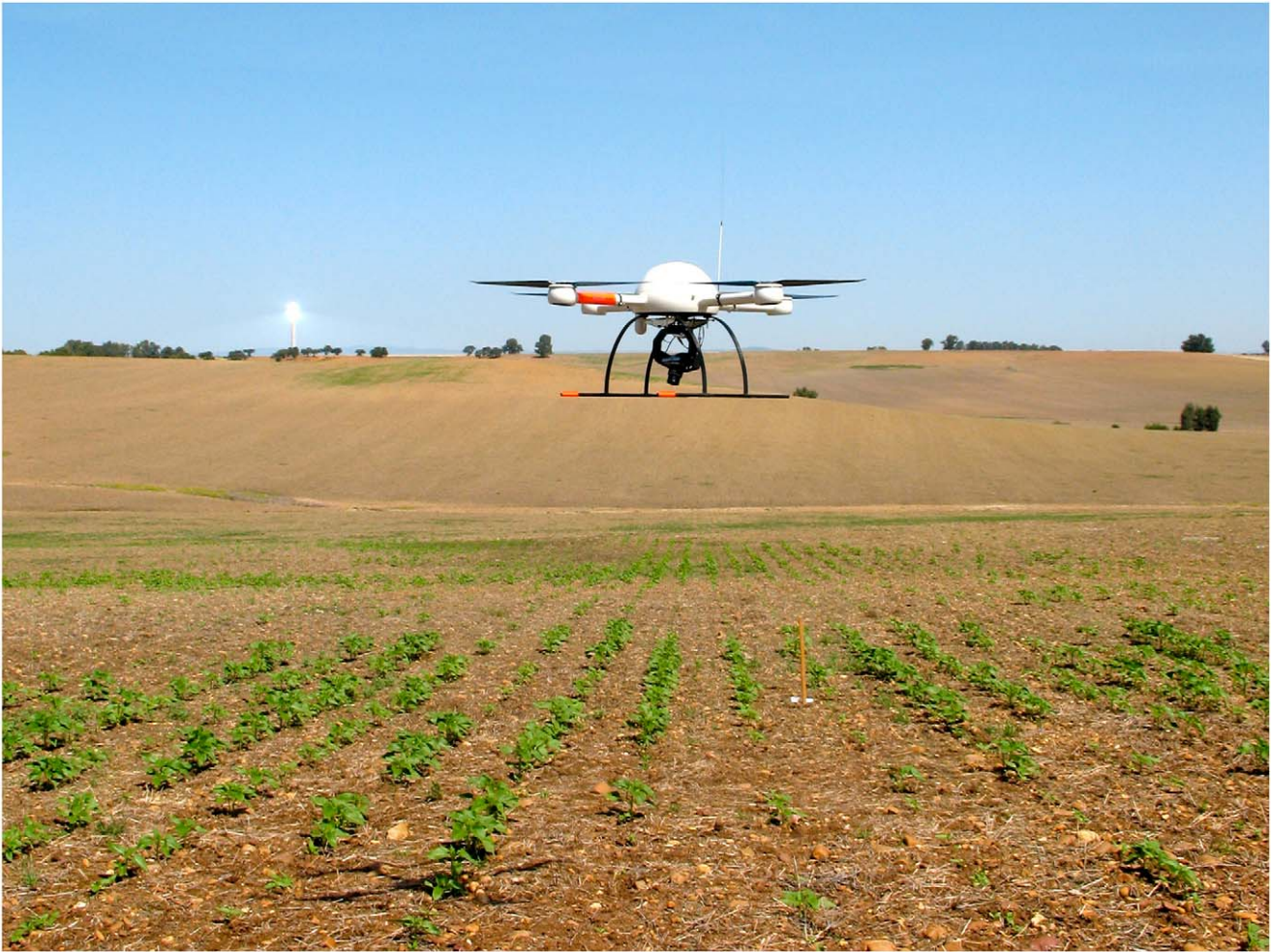
Figure 1. The quadcopter UAV, model md4-1000, flying over the experimental crop-field. doi:10.1371/journal.pone.0058210.g001
