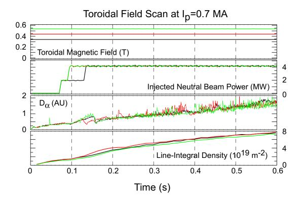
Figure 1: Overview of toroidal field scan at  $I_p=0.7$  MA. Plotted are toroidal field levels (0.35, 0.45 and 0.55 T) along with beam power in the top panel, the  $D_{\alpha}$  trace in the middle panel, indicating all three  $B_T$  levels were H-mode discharges with small ELMs, and the line-integral density in the bottom panel, showing comparable densities for all three toroidal fields.
