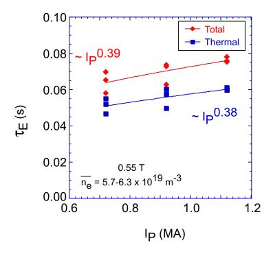
Figure 3: Total (red) and thermal (blue) energy confinement times vs  $I_p$  for the plasma current scan at constant toroidal field, density and heating power.
