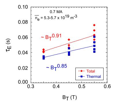
Figure 2: Total (red) and thermal (blue) energy confinement times vs  $B_T$  for the toroidal field scan at constant current, density and heating power.
