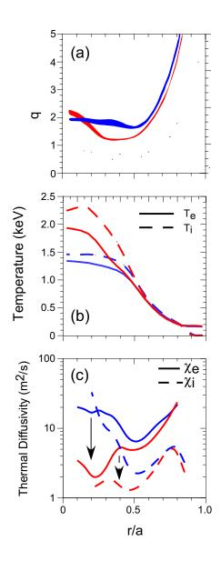
Figure 9: (a) q-profile comparisons for discharge with low central magnetic shear (blue) and strong reversed magnetic shear (red). (b) Electron (solid) and ion (dashed) temperature profiles for discharges shown in (a). (c) Electron (solid) and ion (dashed) thermal diffusivities for the discharges shown in (a).
