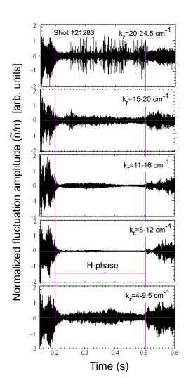
Figure 14: Normalized density fluctuation amplitudes  $\tilde{n}_e/n_e$  as a function of time for a discharge that transitioned from L- to H-mode, and then back to L-mode. The density fluctuations were measured by a tangentially viewing microwave scattering diagnostic. The diagnostic measures  $k_r$  from the upper ITG/TEM range up to the ETG range.
