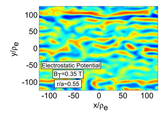
Figure 13: Results from a non-linear fluid calculation with finite Larmor radius corrections of the 0.35 T discharge at r/a=0.55. The calculation shows the formation of radial streamers with radial extents of  $200\rho_e$  (~ 2 cm).
