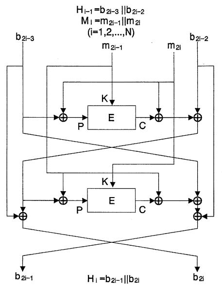
K: Key input, P: Plaintext input, C: Ciphertext output
