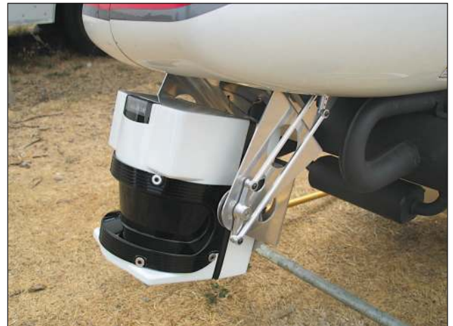
Figure 3. A laser scanning device mounted on an actuated mounting platform.
