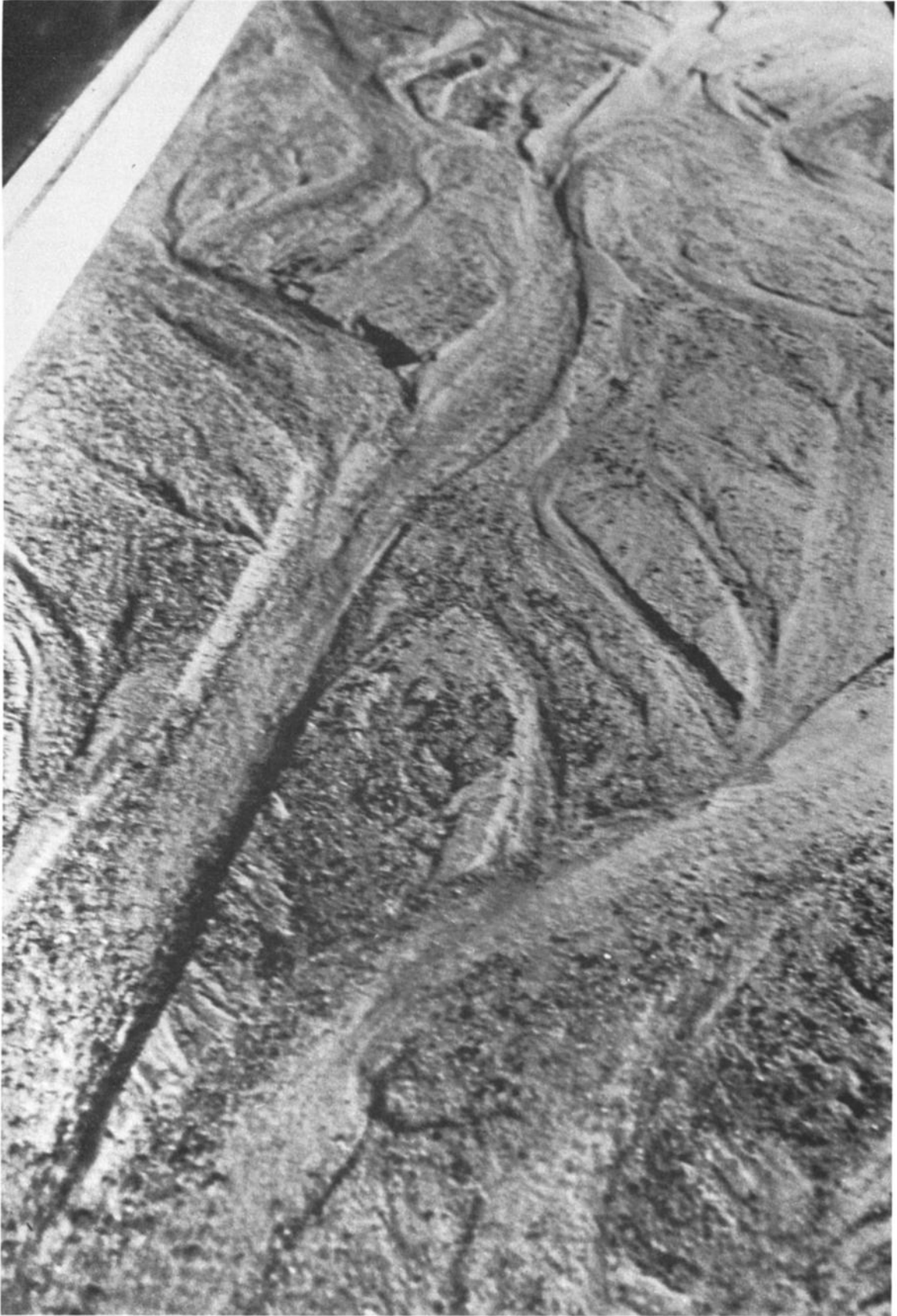
Fig. 5c. View of the valley flat of the Series 2 model experiments. The flow is off. The black particles are coal tracers.
