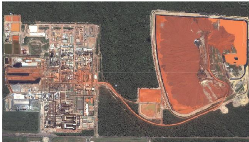
Figure 1: Picture of an industrial plant of bauxite processing showing the red mud deposit (Souza, 2010).
