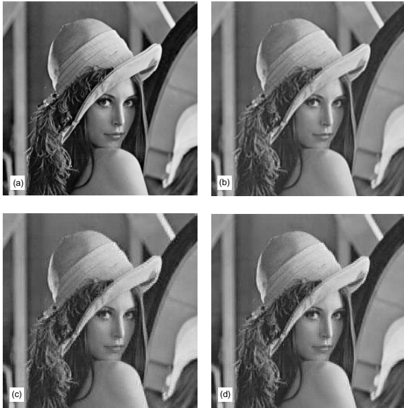
Fig. 10: (a) The original image of Lena, the decompressed images of Lena using (b) the DCT, (c) the proposed transform, and (d) the WHT using 20 transform coefficients.
