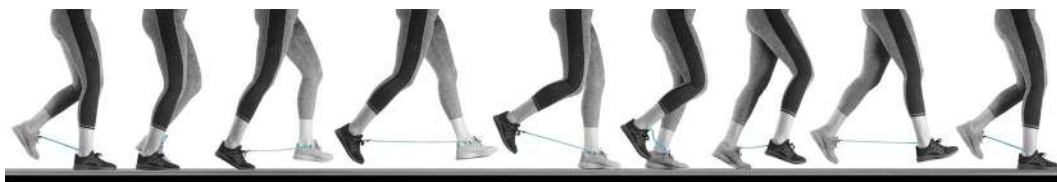
Fig. 3. Time-lapse photographs of a runner using the exotendon. The length of the exotendon is tuned so that the device is long enough that it does not apply forces when the feet cross each other and does not break when the feet are far apart, yet short enough that it does not become entangled when the feet pass each other. Images span one complete gait cycle.
