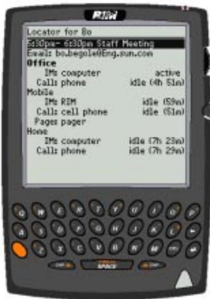
Figure 7. The Contact Locator (shown on a RIM) shows a salient appointment, an e-mail entry, and awareness information on all devices in each locale.
