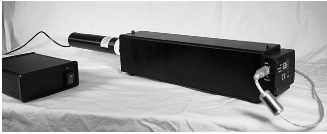
FIG. 1. From the left, the regulated power supply for the laser, the HeNe laser tube extending out of the optical apparatus, and the camera attached to the right side of the apparatus. The housing is a precision-machined aluminum box, painted matte black and optically sealed.
