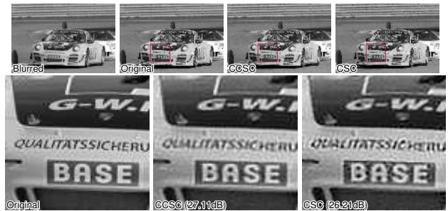
Figure 10: Deconvolution results using 2D filters for the Car example. Top row show from left to right: (a) Blurred image, (b) Ground Truth, (c) CCSC, (d) Conventional CSC. Bottom shows insets from (b-d) respectively. In darker regions such as the car text conventional CSC hallucinates features which are not present resulting in poor deconvolution results.
