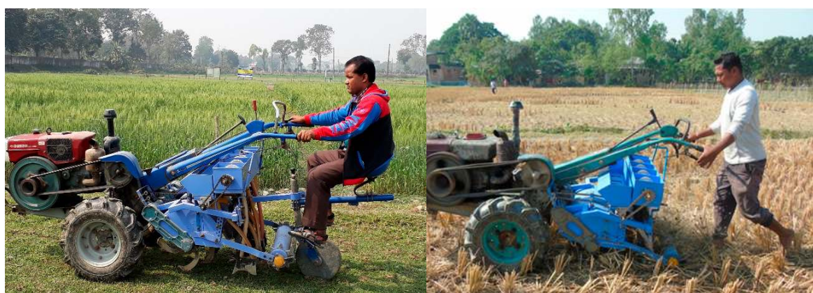
Figure 5. VMP, attached to a 2WT: in transportation mode (left); and field operation mode (right).
