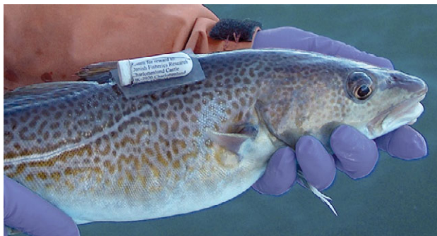
Figure 6: An Atlantic cod ( Gadus morhua ) carrying a data storage tag that records pressure, temperature and salinity. Photograph: Stefan Neuenfeldt, DTU Aqua.
