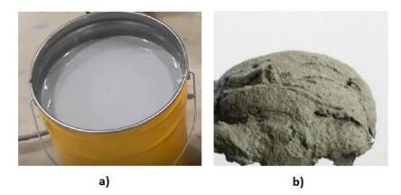
Figure 8. Example of the matrix in the laminate: (a) epoxy resin and (b) cement.
