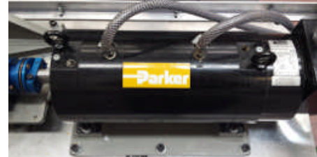
Fig. 17. Commercial high-speed interior permanent magnet machine used for spinning the PMSM under test.
