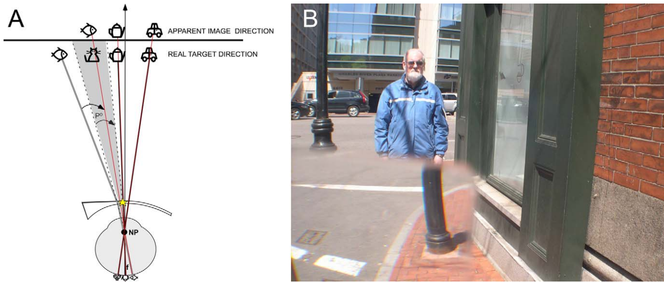
Figure 1. Apical prism scotoma. (A) Schematic ray diagram of the apical scotoma of a sector prism. The apical scotoma occurs between the last undeviated ray and the first light ray which is deviated by the prism (prism apex highlighted by yellow star). The angle between these two light rays is equivalent to the prism power in degrees. In this example, the cat is not visible through the prism, since it is located within the prism's apical scotoma, indicated by the gray shading. (B) Photograph taken with a 30\Delta prism with base to the left covering most of the lower left quadrant of the frame. The prism extends the camera's field of view to the left, revealing crosswalk left of the lamppost, but loses field at its apex, as the lower half of the man is now missing. Had the prism extended the full height of the image, the man would be lost completely to the apical scotoma. The aperture of the camera lens creates vignetting at the prism edges.
