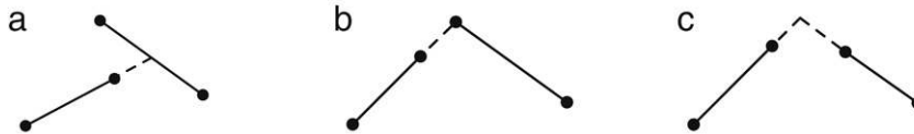
Fig. 25. Geometric update for extending edges: (a) one edge is extended, one vertex must be inserted; (b) the extension corresponds to an existing vertex; (c) both edges are extended.
