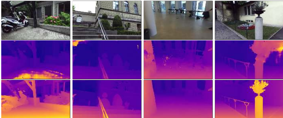
Fig. 4. Disparity estimation results in real scenes different from training. Top: input left image, Middle: feedforward results, Bottom: results with consistency guided refinement. Note that refinement can significantly improve drastically incorrect predictions.
