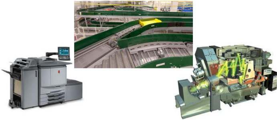
Figure 1.2: Modern mechatronic products, requiring multi disciplinary design approaches. An Océ print engine, a Vanderlande baggage handling system, an ASML ultraviolet lithography concept.
