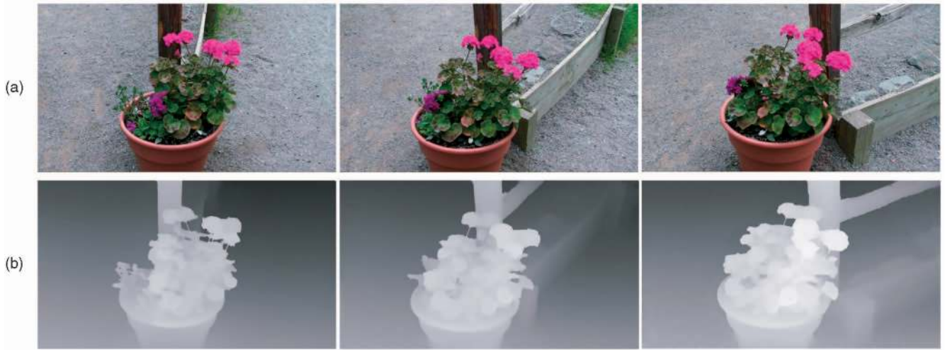
Fig. 10. “Flower” sequence. (a) Extracted frames from the input sequence. (b) The estimated depth maps.
