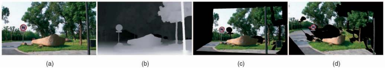
Fig. 9. Novel view synthesis with the recovered depth maps. (a) One frame extracted from the “Road” sequence. (b) The estimated depth map. (c) and (d) With the depth information, we build the texture-mapped scene surface, and synthesize new images with different view angles.
