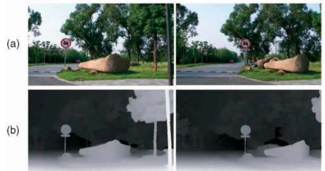
Fig. 8. “Road” sequence taken by a hand-held DV camera moving along a road. Row (a) shows a few frames, and row (b) shows the correspondingly estimated depth maps.
