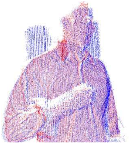
Fig. 11. Merged camera A (red) and B (blue) points clouds resulting from unwrapped phases of Fig. 9.
