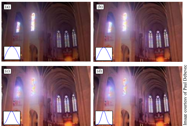
Figure 4. Variation of parameter c_1 . We increased the parameter c_1 for the standard deviation of the Gaussian in intervals of 2.0 as (a) 1.0, (b) 3.0, (c) 5.0, and (d) 7.0. c_1 = 3.0 is a good compromise between contrast compression and loss of detail in bright areas. Of course, a user may have a slightly different individual preference. Inset : plot of weighting w(x) .
