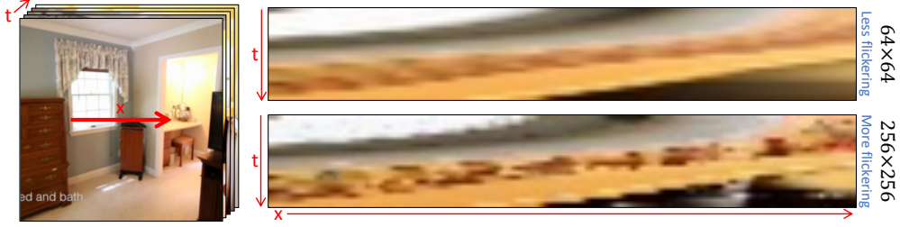
Figure 8. X-T slice visualization. We visualize the x-t slice of the low-resolution ( top ) and high-resolution ( bottom ) videos. The flickering mainly comes from the super-resolution stage.
