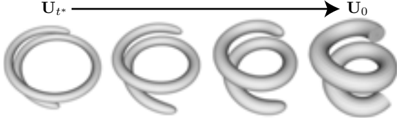
Figure 6: We evolve the intersection-free surface obtained with cMCF to a one that is similar to the input surface intrinsically, but without self-intersections.
