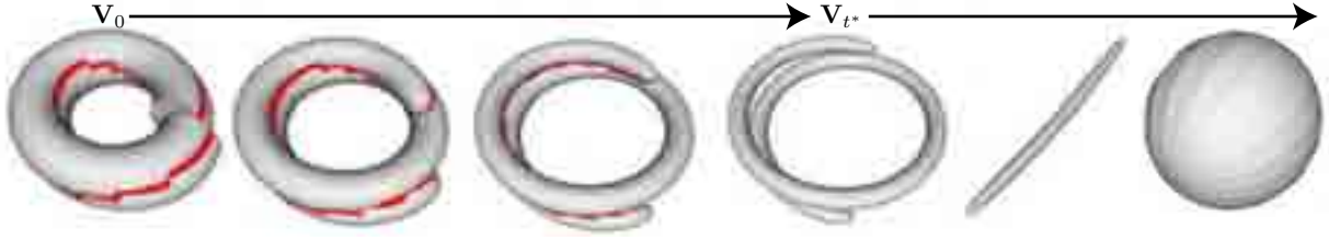
Figure 5: We evolve a self-intersecting surface (intersections are shown in red) with the conformalized Mean Curvature Flow. After some time t^* the surface reaches a self-intersection free state. The limit is a conformal mapping to the unit sphere.
